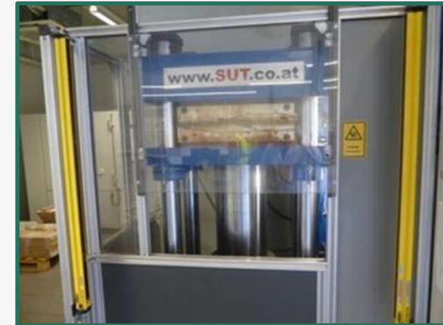
4 th process step - Hot pressing
