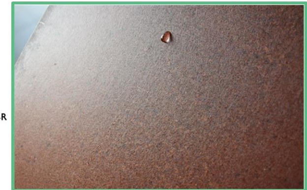
Powder-coated paper substrate using modified lignin
