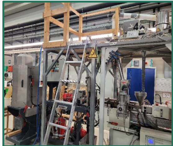
1 st process step - Compounding
